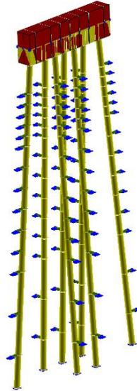
**Fig. 6.** Batter Pile Alternative With 9 Piles
