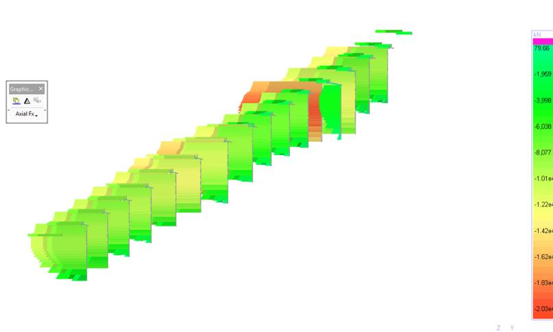
**Fig. 5. Axial Load Distribution In Barrettes/Caissons Under Service Load Combination**
