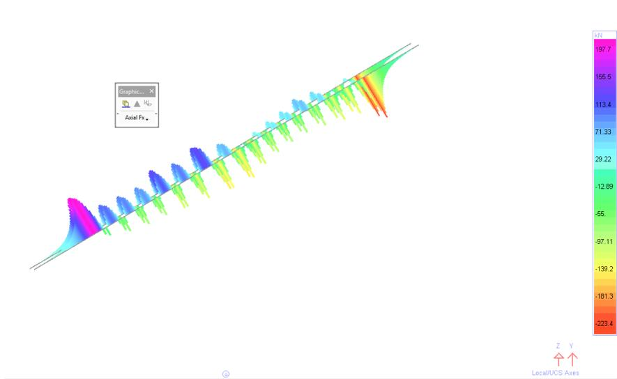
**Fig. 4. Rail Forces Under a Temperature Rise of 35 •**
