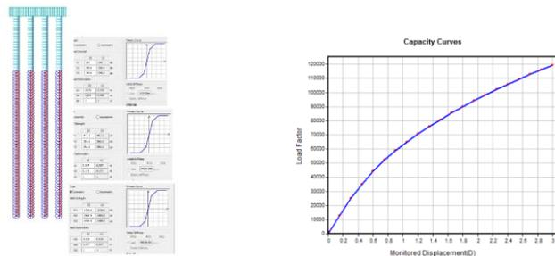
Fig. 11. Pile foundation modelling for pushover analysis
