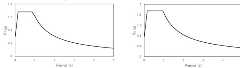
Fig. 7. Design spectrums (Tr=1000 yrs and 2475 yrs)
