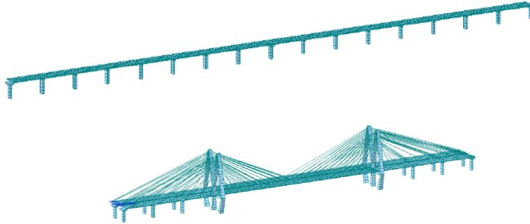
Fig. 8. Structural models of approach bridge and cable stayed bridge
