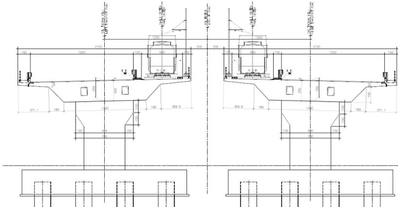
**Fig. 5.** Typical section of the piers
