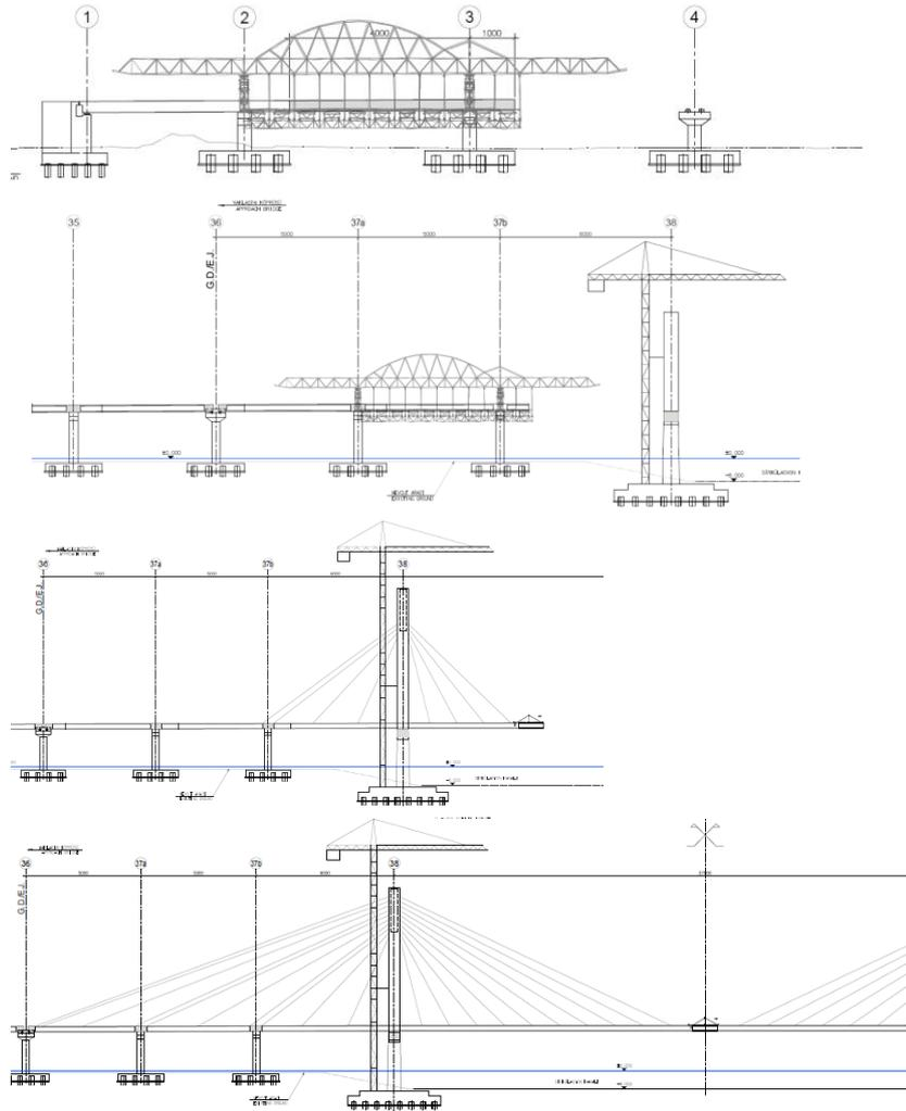
**Fig. 13.** Construction stages of deck
