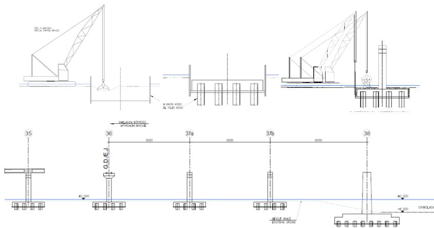
**Fig. 12.** Construction stages of substructure
