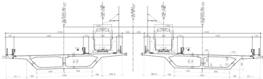
**Fig. 4.** Typical cross section of the deck
