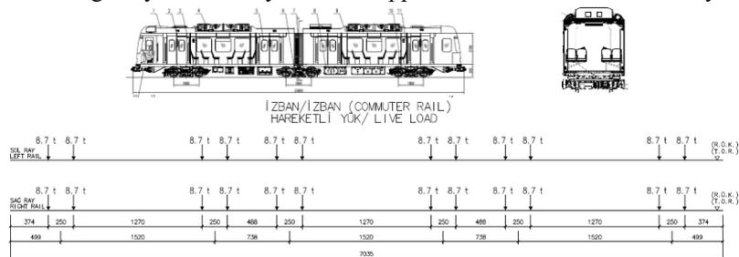
Fig. 6. Rail system loads
