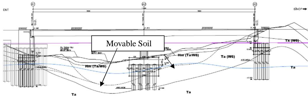
Figure 4. Foundations of the Idemli-2 Viaduct are Located on Relatively Shallow Landslide Prone Regions
