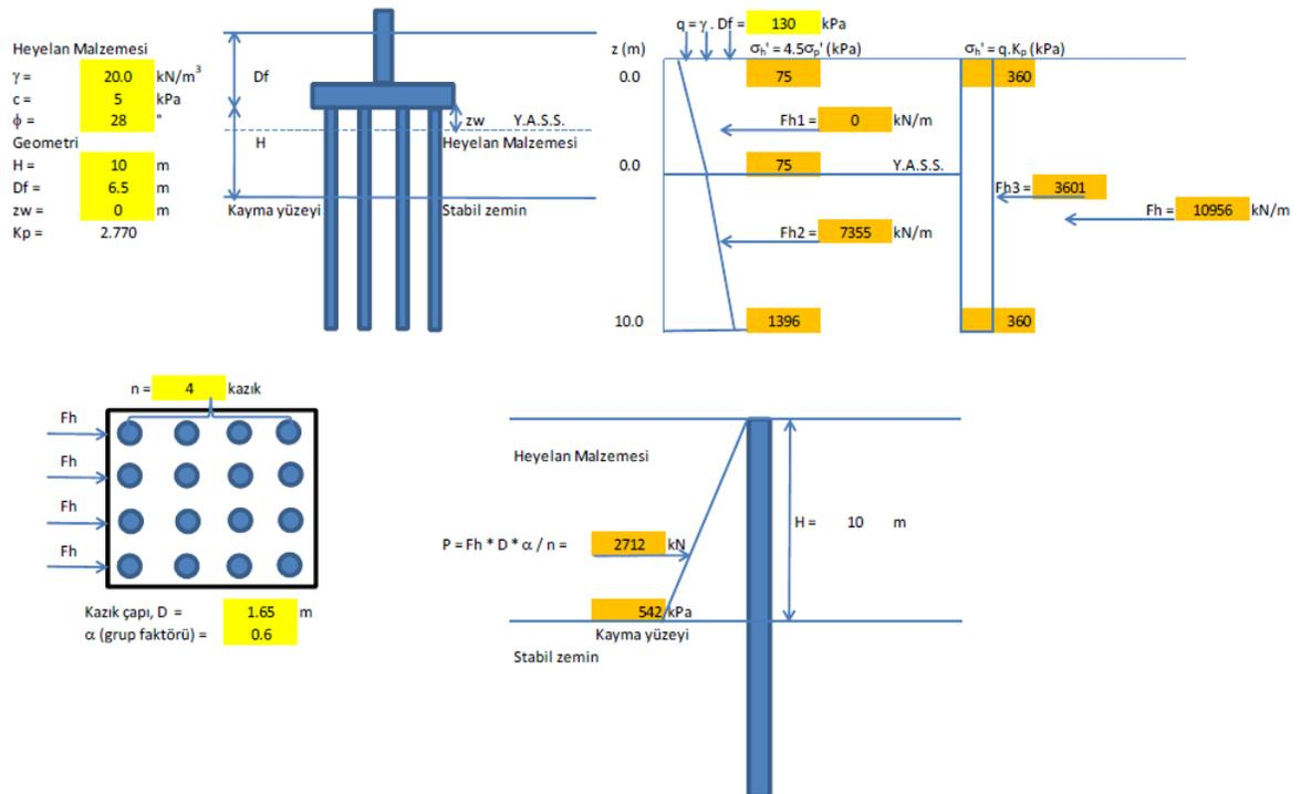
Figure 8. Representation of the Thrusts Applied By the Movable Soils to the Pile System
