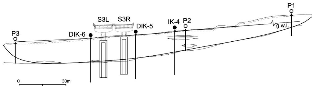
Figure 2. An Application for Design of a Bridge Foundation In a Landslide Area- (P1, P2, P3, DIK5, DIK6, IK4 indicates inclinometer positions) (Nossan et.al, 2009)
