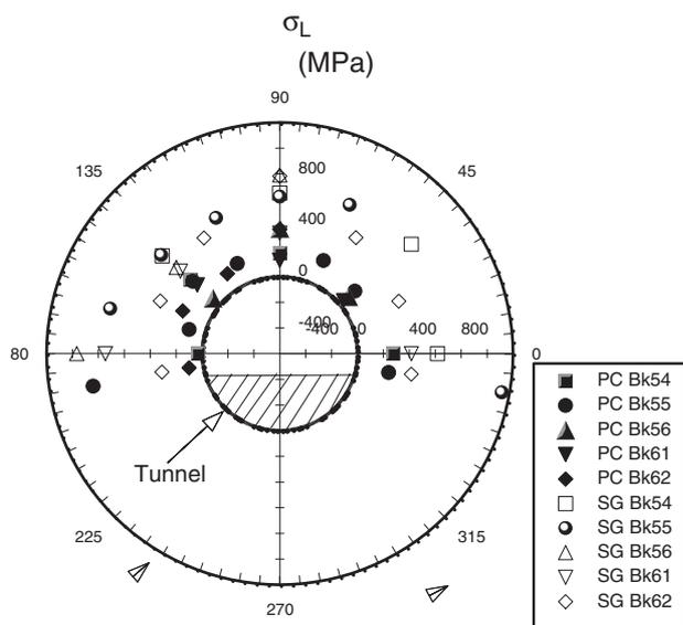
Figure 4. Earthquake induced radial stresses (kPa) on inner lining from pressure cells and embedded strain gauges.
