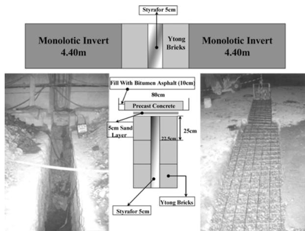
Figure 7. Detailed seismic joints in the monolithic invert.
