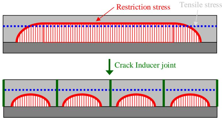
Figure 7. Effect of crack inducer joint
