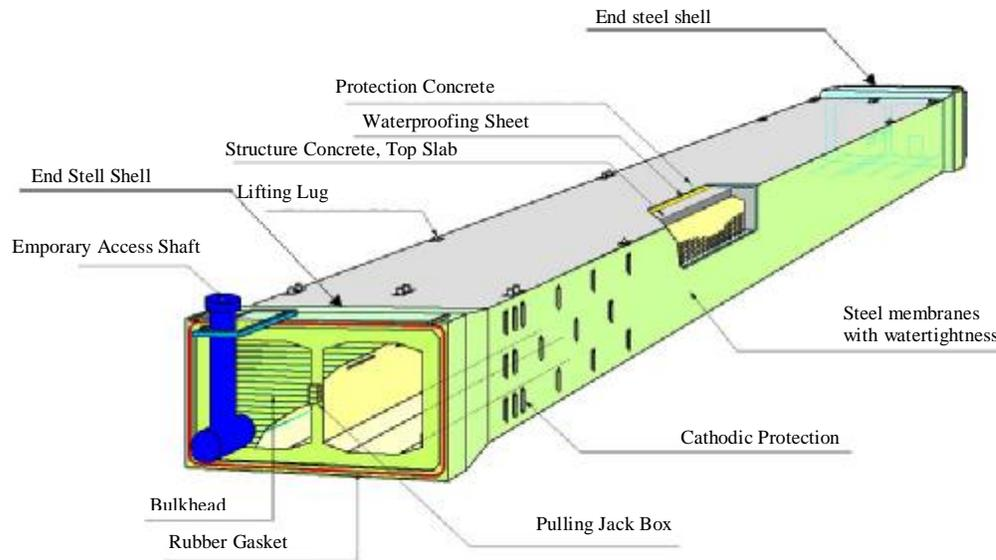
Figure 2. Typical Section View of Immersed Element
