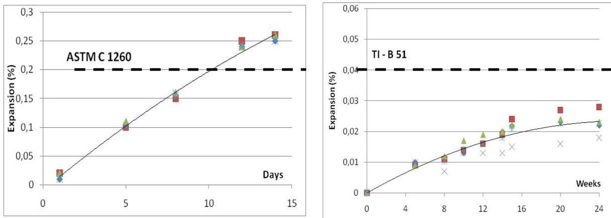
Figure 3. Expansion test results of natural sand
