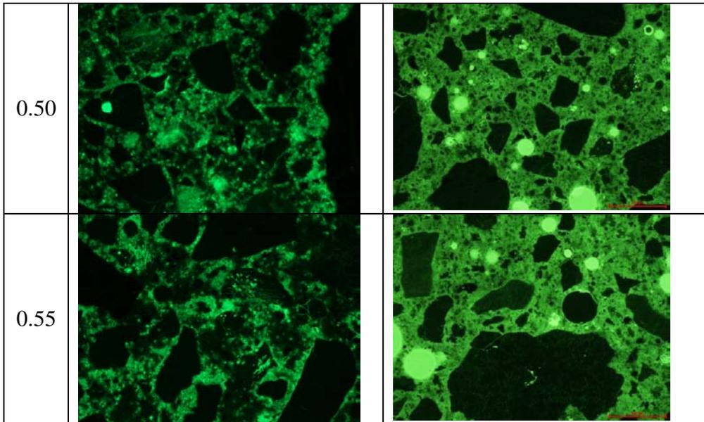
Figure 2. Effect of water-to-cement ratio and cementitious material content on the UV light intensity under polarising microscope (x50).
