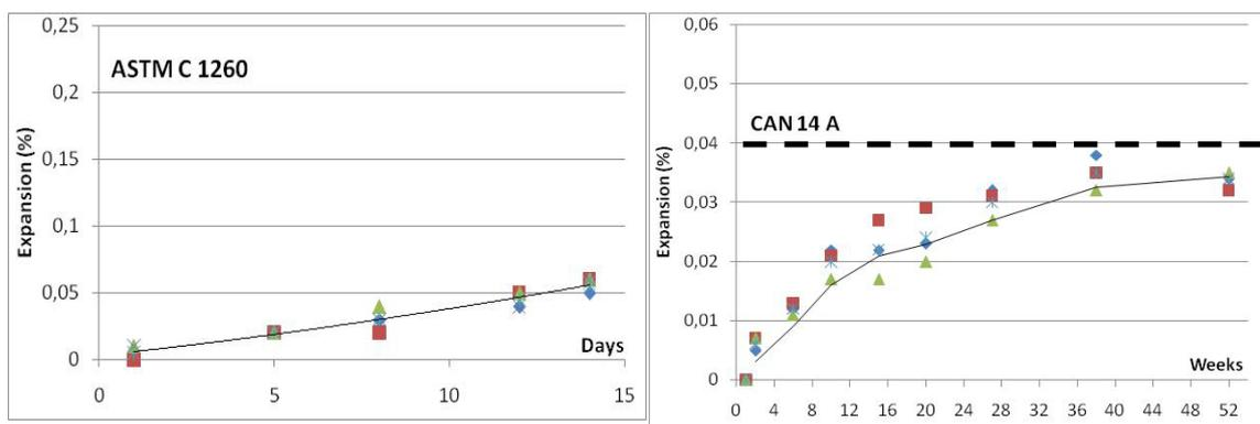
Figure 5. Expansion test results of crushed sand
