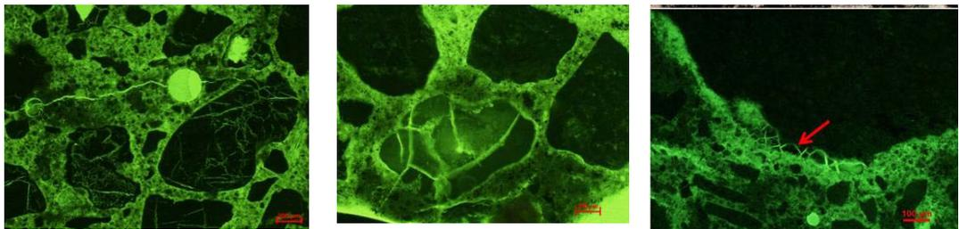
Figure 4. UV light views of reacted porous sandstone (left, x50), porous chert (middle, x100), biomicritic limestone with disseminated secondary microquartz (x50).
